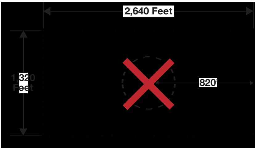
\* These setback illustrations assume minimal tower spacing of three rotor diameters or 690 feet and system height of 410 feet on a rectangular 80-acre parcel. The same assumptions on a square 160-acre parcel would allow installations of 11, nine and five turbines, respectively.
